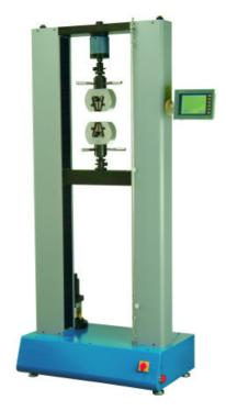
This tester has been wide used in electronic, tape, textile...industries. With a multi-function indicator, which can provide max and elongation, value and these values can be printed.
